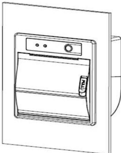
**Step 2:Turn the printer cover and turn the screws on both sides clockwise until the screws are locked so that the product is fixed OK**
