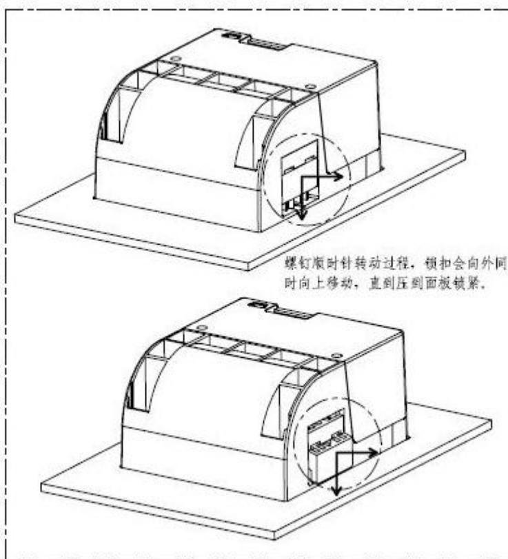
**Noted:** Screw clockwise rotation process, the lock will move outward at the same time upward, until the panel is pressed to lock tight.
