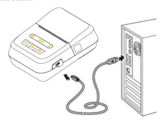
Note: USB has two types: virtual serial port and print port. Default is print port.
