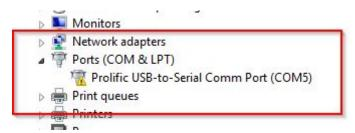
For instance: If you unplug the USB cable, above icon disappears, and it appears when reconnected. That means COM7 is the port which connects printer to computer.
