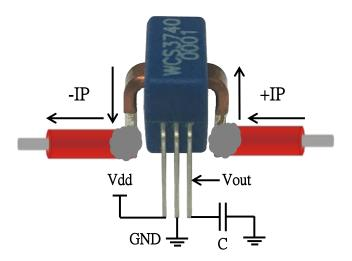
Capacitor C(0.01uF~0.1uF) is recommend to be connected between Vout and GND to reduce output noise.
